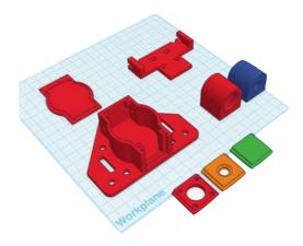
The case went through a number of iterations, and prints. The above design is the latest version but seems to always be in a state of flux. The T clip you see in the design enables the dipole centre to be attached to a painters pole or slid down a fibre mast.
